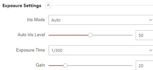
Figure 2-3 Set Exposure Time According to Vehicle Speed
