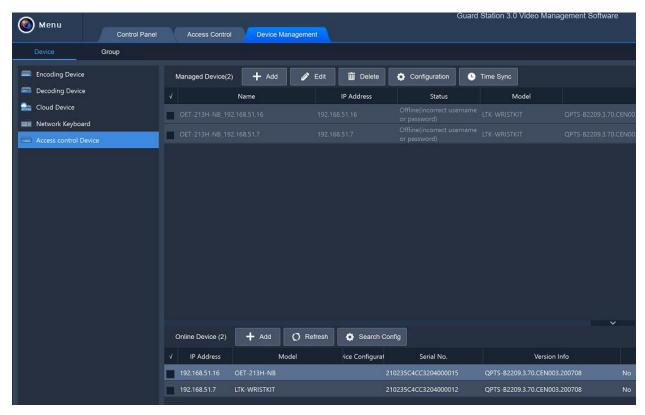
Note 1: IP discover tool is under "Device Management" – "Access Control Device"
