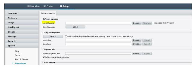
Upgrade Step 1 first, then upgrade step 2. Device will reboot between steps 1 and 2.
