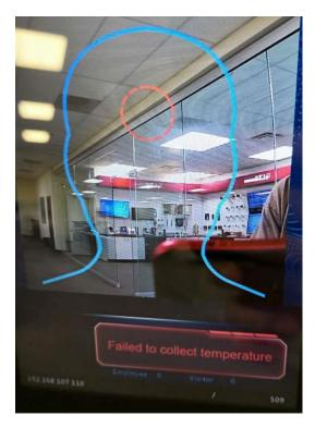
When customer sees an outline as the pic above shows, check the wiring to the wrist module.
