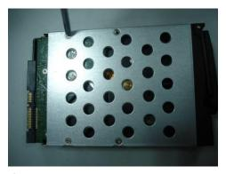
①Use 4 screws to secure the HDD
