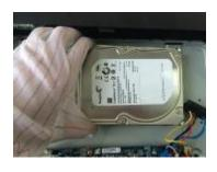
④ Place the HDD in accordance with the four holes on the bottom of the chassis.
