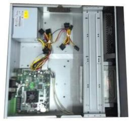
7 Put the bracket back. Please adjust the CD-ROM to the proper position so that the button of the front panel is directly facing the pop-up button of the CD-ROM.
