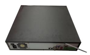
① ①Use the screwdriver to loose the screws of the rear panel and then remove the front cover.
