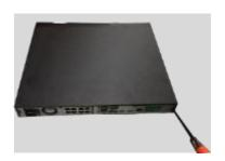
⑤ Put the cover in accordance with the clip and then fix the screws on the rear panel and side panel.
