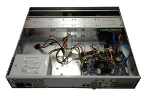
3 Connect to the HDD data cable to the main board and the HDD port respectively. Loosen the power cable of the chassis and connect another end of the power cable to the HDD port.
