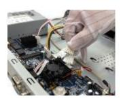
② Connect the one end of the HDD data cable and the power cable to the mainboard.
