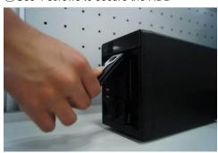
③Pull the HDD knob up when you put the HDD into the box in case the knob buckle may strike the front panel.
