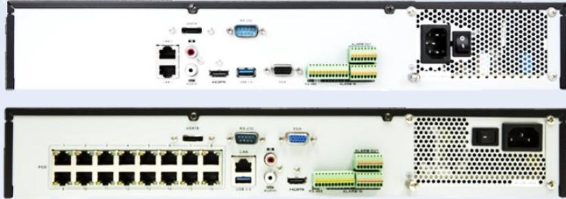
For the regular NVRs without PoE are usually supporting more than 16 channels. (32ch,64ch,128ch,256ch)
