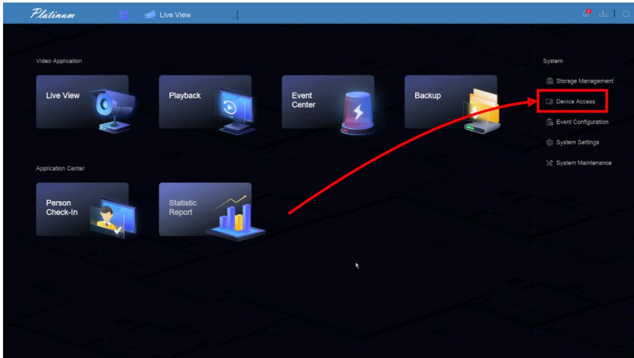
In NVR5 firmware, PoE channels can not be edited to become manual add channels, they must be disabled by accessing the “PoE Settings” section in the menu on the left side.
