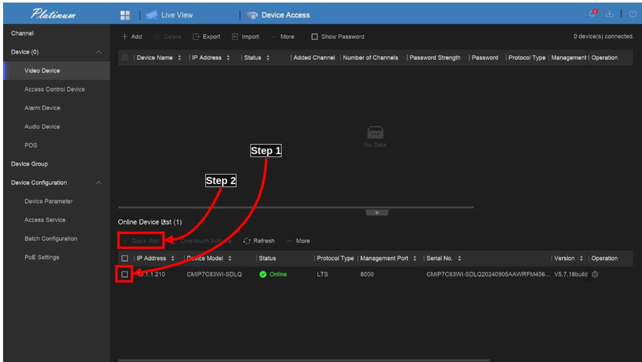
If the IP cameras are not utilizing the same password as the NVRs default channel password, they must be manually added. Click the “+ Add” button near the top under the main menu icon. Type in the relevant information for the IP camera such as IP, port, username, password, etc. Once finished click Add at the bottom.
