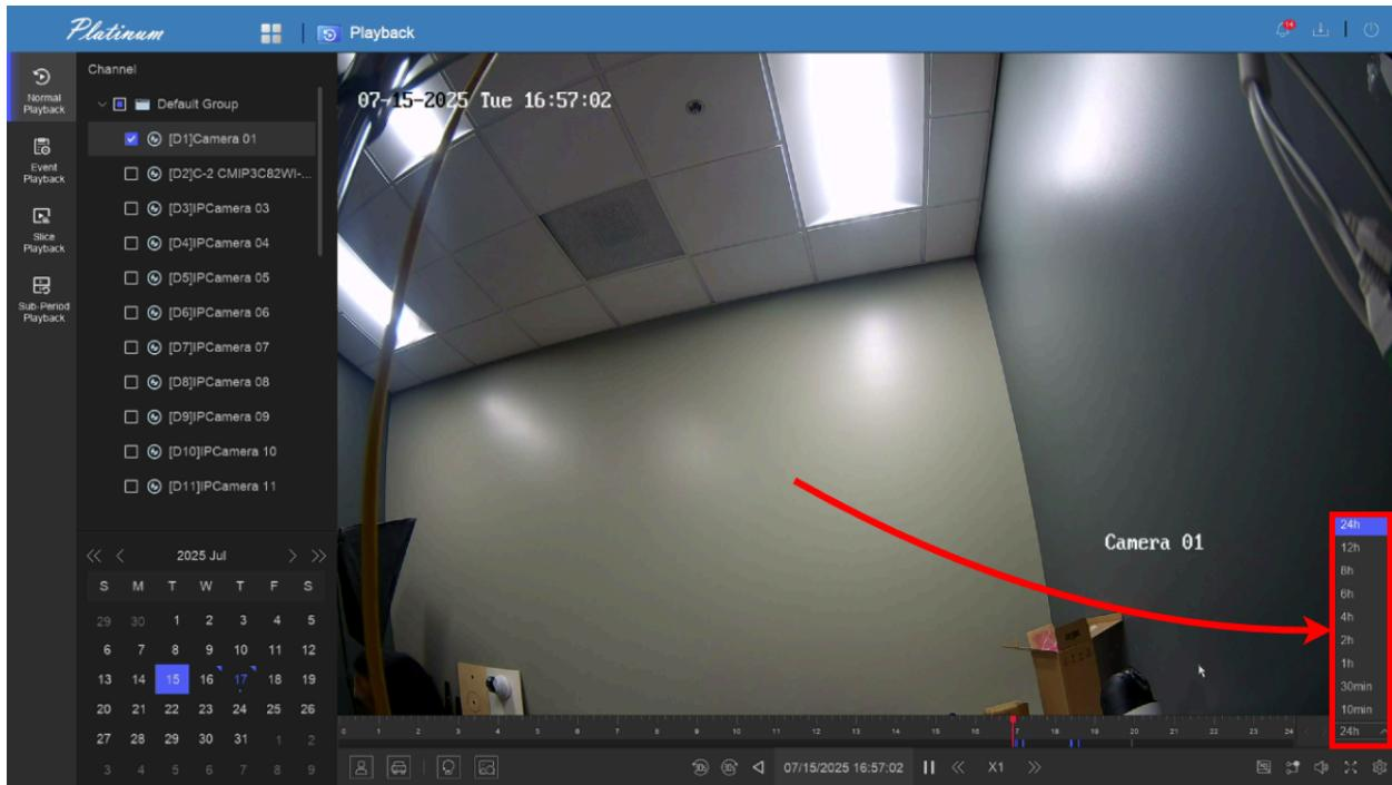
A snapshot will also be shown when mousing over the timeline with the mouse.
