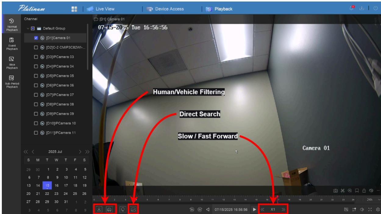
It is possible to have multiple cameras playing back as well. Please be sure to refer to the recorders maximum decoding capability when doing simultaneous viewing. All that needs to be done is to select multiple cameras.
