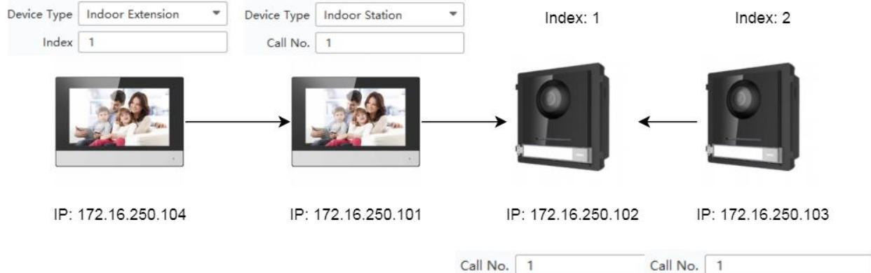
Pushing the button on either the Main or Sub Door Station will ring both indoor stations at the exact same time.
